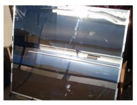
An excellent reflection: the reflected sun is precisely behind the receiver.
