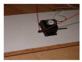
The traction wire is put in a guiding channel made of a bended angle, to reduce its length variation when the position of the collector changes.
