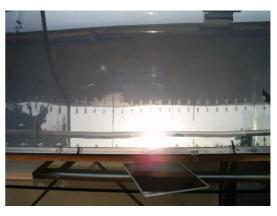
By the way, the above two pictures show an image of the receiver which is still quite straight and regular near the edge of the collector. This image is an important indicator of the optical quality of the collector, and at the same time a difficult one. The reader can compare this to the large number of published pictures of other parabolic troughs, in order to appreciate the quality of this realisation: the others usually give far worse images.
