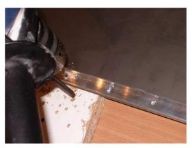
Fasten the side angles on the back using 3mm bolts and washers as shown, one at each side. Check that the tails of the bolts do not exceed the straight line joining the two outer edges of the angle. If they exceed, the exceeding part must be cut off.
