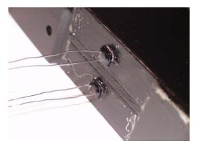
Le the glue dry, then fill the surrounding sace with blu-tack to stop light leaking.
