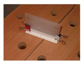
Then glue on the two base pieces. Note that the two 3mm bolt holes on the base pieces must be exactly located on the center line of the assembly, with a tolerance not exceeding 0.2mm. Space should be left above the hole for the head of the bolt.
