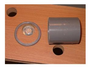
Put the ring as shown, then fix the assembly by epoxy. Close all the gap to prevent water infiltration.
