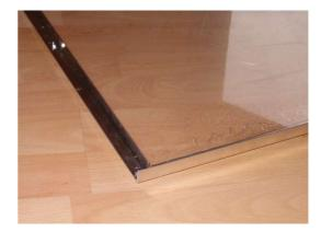
A gap of 2.5mm should be left between the edge of the cover and the vertical side of the end angle. When the cover is assembled, the end reinforcement bar will enter this gap.
