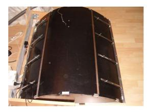
Cut and bend body redressing wires as shown. Here two wires will be enough.
