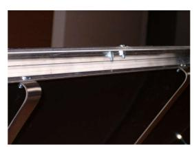
And press down the cover at the ends so that the upper edge of the end reinforcement bar enters into the gap between the edge of the cover plate and the vertical side of the end angle of the cover. Fix the position using adhesive ribbons. Do not apply a more permanent fixation means unless you are sure that you won't need to reopen the box.
