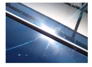
Leaking from the above: some sunbeam appears from above the receiver. It is a partial leaking, in the sense that only a quite small portion of the sunbeam misses the receiver.
