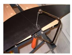
Smoothen the hole with a file, to the point that the bearing can be inserted neither too tight nor too loose.
