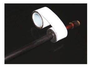
Adjust the wraping such that it just enters into the bearing and is able to turn around, neither too tight nor too lose.
