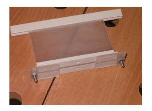
Seal the heads of the bolts with epoxy.
