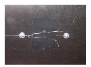
Once the position of the photoelectric detector is adjusted during field test, fix the tail of the two bolts with silicone or lacger, to prevent movement and water infiltration.
