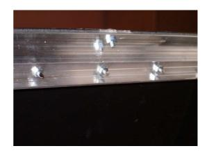
Press down the cover, so that the edge of the back plate reaches the lower surface of the cover.
