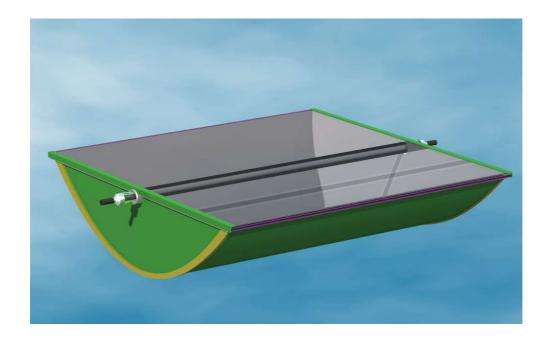
There are two basic choices of the materials forming the collector box. One can either use allplastic plates for the body of the box, or use glass cover plus metal back and ends. The cost and performance of the two choices are very close. For manual work, it is easier to make and to manipulate a plastic box. Therefore our description will be given for the plastic case. But it is easy to adapt the description to glass and metal boxes.
