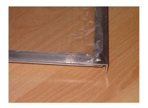
This picture shows the cracking of the cover by the bolts. This phenomenon is quite noticeable when a polystyrene plate is used for the cover. No cracking is observed when a polycarbonate or HIPS plate is used.
