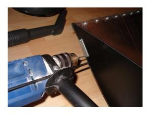
Apply silicone to the joining surfaces, then re-insert bolts and fasten, according to the direction shown in the picture.
