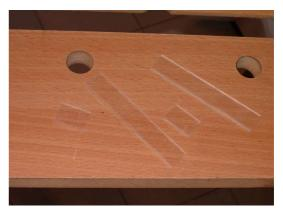
Thoroughly scratch the surfaces of the two longer bars with coarse sandpaper, to create a scattering effect.
