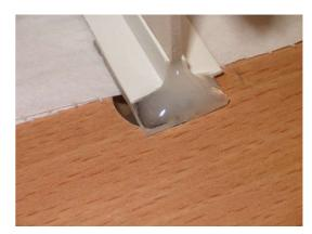
Paint the assembly to black. The surfaces of transparent materials must be carefully blackened in order to prevent interference by leaked lights.
