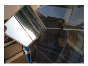
Paper stripes can be put on the cover to check leaking, as a leaking will illuminate portions of the stripes. This is particularly useful for checking leaking coming from the middle portion of the reflective mirror.
