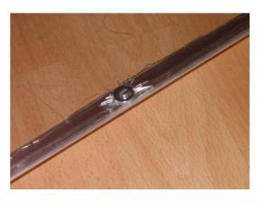
To protect the outer surface of the cover against scratches, the easiest method is to put a thin plastic film on it. The plastic food wrap is good for this, but a thicker one would be better. Care must be taken not to leave air bubbles between the film and the plate. There will be no light loss if there is no air bubbles.
