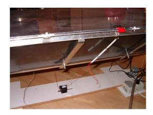
A flexible adhesive ribbon is first wrapped on the output axis of the motor to increase friction.
